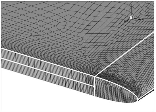
trailing edge discretized with 8, 12, 18 cells
